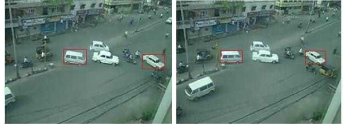
Figure.6. Moving Blobs Identified between Frame 1 and Frame 2 by applying Equation (1)
