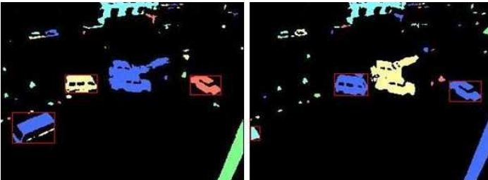
Figure 5 Blob Filtering Constraints Applied over the list of Blobs and Convex Hull Marked over Similar Moving Blobs
